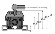
Extensive mounting accessories provide various options for installation. Due to the measuring principle, which is based on the functional principle of an RLC coupling, the linear position sensor is immune to magnetized metal splinters and other interferences.
