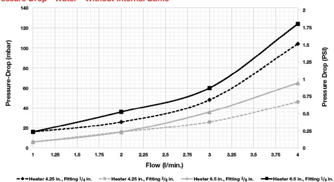
Pressure Drop - Water - Without Internal Baffle
