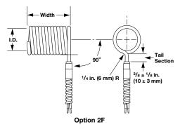
**Note:** Coiling or complex forming of stock heaters will generally result in increased resistance and reduction in wattage below 10 percent tolerance. Please contact factory before specifying power and resistance tolerance for formed cables.
