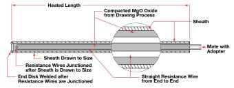
Straight resistance wires are positioned inside a large diameter metal tube. The tube assembly is repeatedly pulled through draw dies until the desired diameter is achieved. Though limited to fixed incremental ohms/foot and without no-heat sections, this **straight wire or drawn cable** construction method allows:
