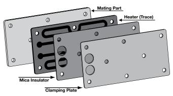
Thick film conduction heaters, designed for clamp-on applications, are supplied as a multi-part assembly: heater, mica insulator, clamping plate and mounting hardware.
