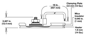
To install, mount the heater to the surface being heated and assemble mounting hardware. Standard measurements of assembly hardware are illustrated in the *Termination Assembly* drawing above. Please refer to the *Installation and Maintenance Manual* (316-42-32-1) that is supplied with the heater for proper mounting instructions.
