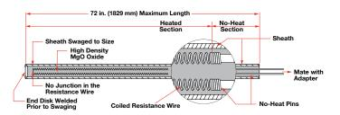
Resistance wire wound into a small coil is loaded into insulating cores, then into metal tubing and swaged to final size. This construction method is called **coil wire or parallel coil.**
