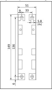
Fig. 22.1-6 Wall/panel mounting, side view
