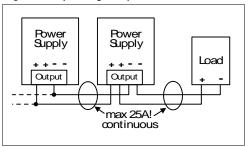
Fig. 12-2 Using distribution terminals
