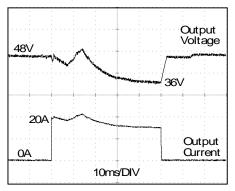
Fig. 23-3 30A peak current for 12ms, typ.
