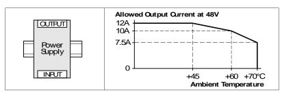
Fig. 23-8 Mounting Orientation B (Upside down)
