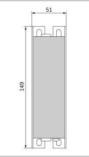
Fig. 22-5 Hole pattern for wall mounting
