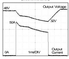
Please note: The DC-OK relay might trigger when the voltage dips more than 10% for longer than 1ms.
