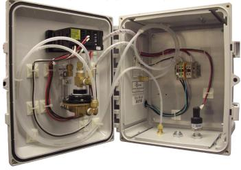
Pressure in the tube is proportional to the depth of the liquid over the outlet of the tube if the liquid density is constant. Air
